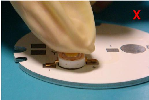
Figure4. Do not press (or puncture by tweezers)on the silicone lens.
